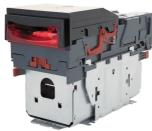
**Bill validator Innovative Technology NV9** - ccTalk communication interface, can recognize up to 16 different banknotes; inhibit for individual banknote and global acceptance; fault detection; public software for setup and configuration; integrated stacker for 300 or 600 banknotes.
